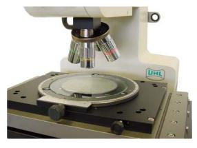
\* Reduces the maximum specimen height to 115 mm
